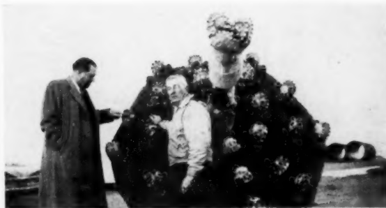
CUTTER TEETH are checked on big bit by Paul Wolff, Kerr-McGee's chief engineer, and Jack Patton, tool pusher.
